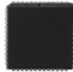
52-LEAD PLCC (FN) (50 mil PITCH)
