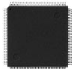
160/144/128-LEAD QFP (FT) (0.65/0.65/0.80 mm PITCH) (28x28 mm)
